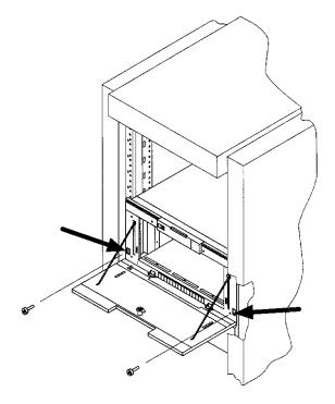
4. Slide the library out of the rack so that it is in the fully extended position.
